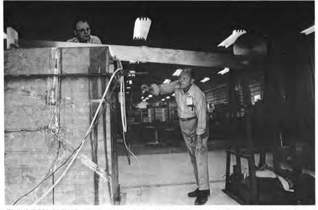
TAKING IT FOR GRANITE — This four-ton hunk of granite is being sawed in two with an ingenious saw devised by Howard Austin (1124), left, and Frank Dain (1126). Saw consists of blade with diamond cutting edge, electric motor and eccentric drive wheel. Cut took a week's sawing. Blocks will be used in study to determine effects of nuclear wastes buried in underground granite.
